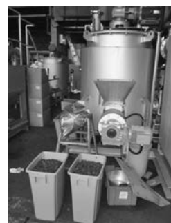
Photo. 1 Equipment used in drying wine pomace. Indirect Heating Type Vertical Dryer, manufactured by Kyoritsu, Inc. (capacity: 3m 3 ).
