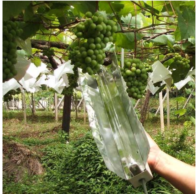
Fig. 1 Simplified device for UV-C irradiation of grape cluster on vine.
